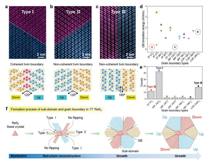
**Figure 3.** Formation of subdomains and GBs in CVD-grown  $\text{ReS}_2$  by reconstruction of Re4-chains. High-resolution ADF-STEM images of a) type II, b) type II, and c) type III GBs seen in CVD-grown  $\text{ReS}_2$ , given below each STEM image is the corresponding structure model. d) DFT-calculated formation energy and e) statistical frequency of the different types of GB. f) Schematic diagram showing the formation process of subdomains and GBs during  $\text{ReS}_2$  growth.
