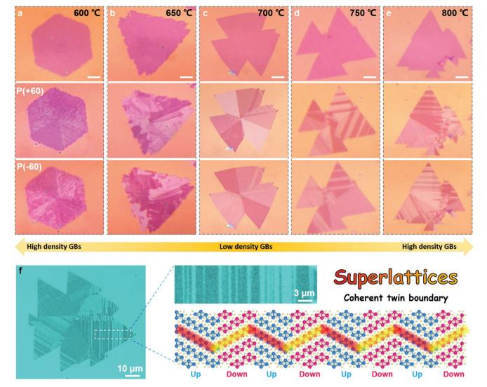
Figure 4. Thermodynamically modulated GB formation in CVD-growth of ReS<sub>2</sub>. OM and POM images of monolayer ReS<sub>2</sub> grown at different temperatures: a) 600, b) 650, c) 700, d) 750, and e) 800 °C. f) Colored POM image of a ReS<sub>2</sub> domain grown at 800 °C and the corresponding structure model.
